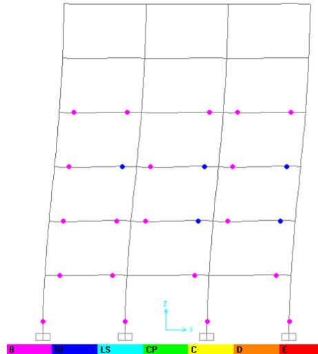
figure III: Hinge status at target displacement
