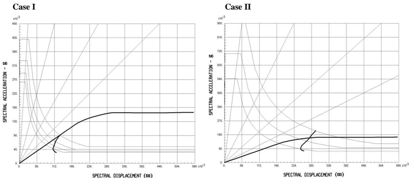
Figure II (a,b,c,d): Target Displacement Results
